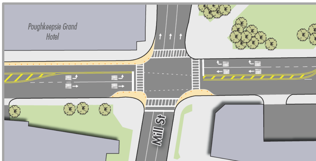
Figure 6: Intersection of Civic Center Plaza and Mill Street in a two-way Market Street scenario.
